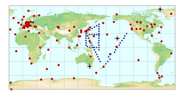
Figure 6: Current configuration of the comprehensive WMO GAW network for CO<sub>2</sub>-based data contained at the WDC for Greenhouse Gases in Japan. Red dots represent in-situ measurements, orange diamonds denote aircraft measurements, and blue triangles are ship measurements. Crosses show main inter-comparison sites. The network for CH<sub>4</sub> is almost identical (Source: WDC-GG).
